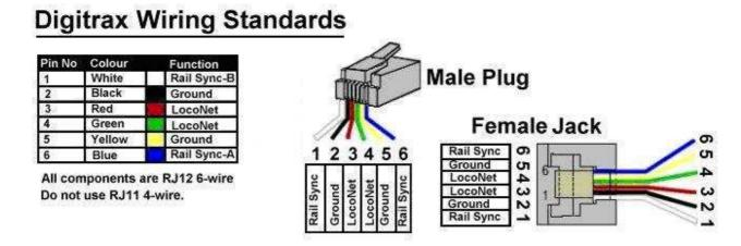
Note the relationship between the Pin Number, the colour of the wire inside the cable and the function. If you look at the front of the male plug, you will see that the White wire (Pin 1) is on the left, and the Blue wire (Pin 6) is on the right side. If you look at the front of the female jack, you will see that the White wire (Pin 1) is on the right and the Blue wire (Pin 6) is on the left side.
