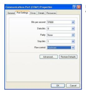
For good functioning of the LocoBuffer the "Flow control" must stand on "hardware" for the RS232 version.
