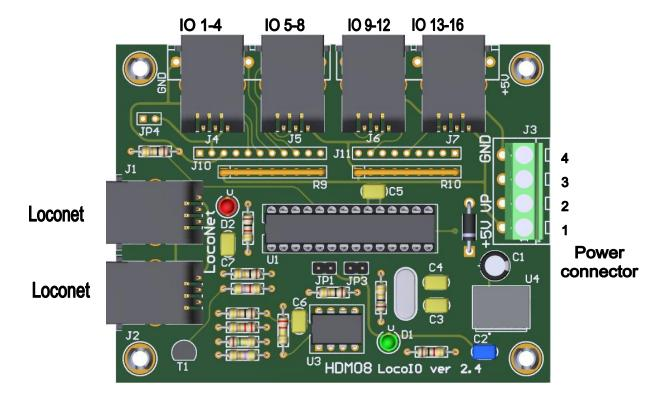
Possibility to make wire connections with PCB connectors J8 and J9 or with pin connections J10 and J11
