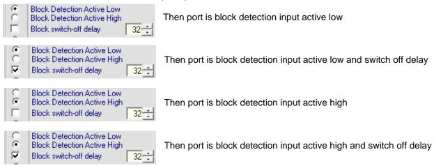
Remark: The switch off delay depends on the established blinking rate.
